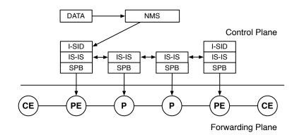
Figure 10: Provisioning a DVPN using SPB.
