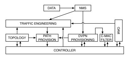
Figure 8: Interactions between application components to implement DVPNs.
