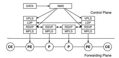
Figure 5: Provisioning a DVPN using MPLS.
