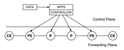
Figure 7: Provisioning a DVPN using OpenFlow.
