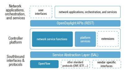
Figure 9: The proposed OpenDaylight architecture.
