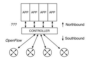
Figure 6: Architecture of SDN and OpenFlow.
